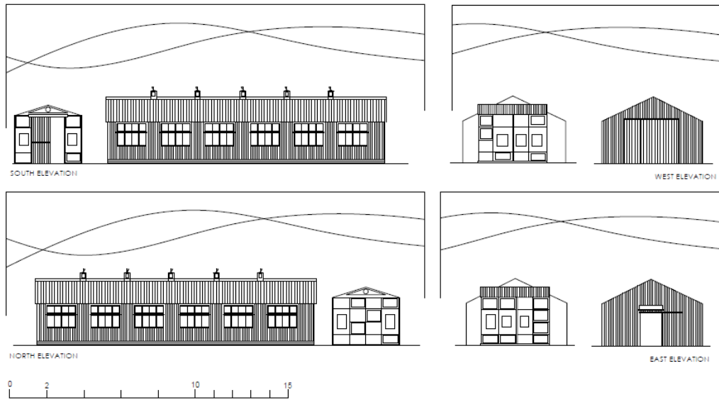
Fig 3. Elevations of demolished stable and the barn
